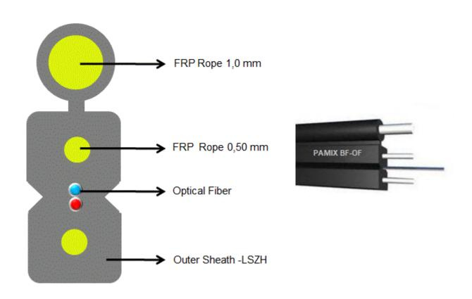
Fiber Type Attenuation at 1310 nm Attenuation at 1550 nm SM 9/125 (G.657 A2) Max. 0.40 dB/km Max. 0.25 dB/km
