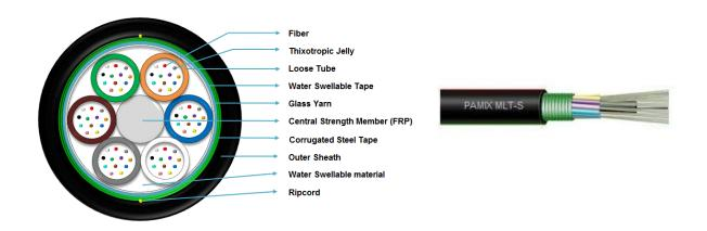
Fiber Type Attenuation at 1310 nm Attenuation at 1550 nm SM 9/125 (G.652.d) Max. 0.35 dB/km Max. 0.21 dB/km
