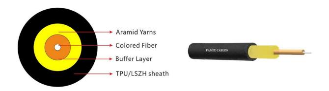
Fiber Type Attenuation at 1310 nm Attenuation at 1383 nm Attenuation at 1550 nm SM 9/125 (G.657 A1/A2/B3) Max. 0.36 dB/km
