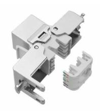
PAMIX Elite keystone jack is a CAT6A RJ-45 female, 4PPoE can deliver up to 90 Watt at PD side with 4 energized pairs, shielded with dust cover. It provide excellent voice, data and video signal transmission. It supports 10G Ethernet application, frequency up to 500 MHz. Its 360° shielding minimizes EMI/RF noise and alien cross talk. Dust cover was precisely designed and fixed to protect internal contacts and keep them clean. Its' one way fixing cap prevent installers' incorrect wiring.
